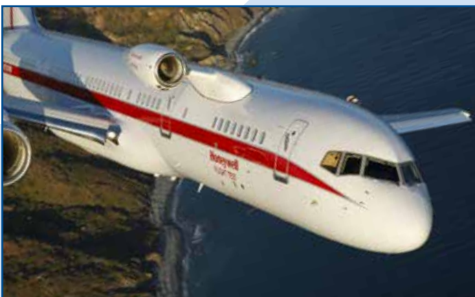
New Business Jet Turboman Mounted on Testbed Fairing Built by Park
