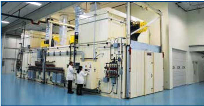
12 Ft. by 8 Ft. by 45 Ft. Dual-Zone Oven
