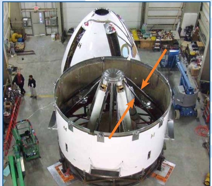
SIGMA STRUTS on NASA's Max Launch Abort System ("MLAS") test vehicle for the Orion Space Program. The struts indicated by the arrows are 11 feet in length.
