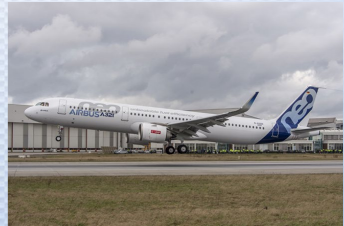
Airbus A321neo with CFM LEAP-1A Engines
