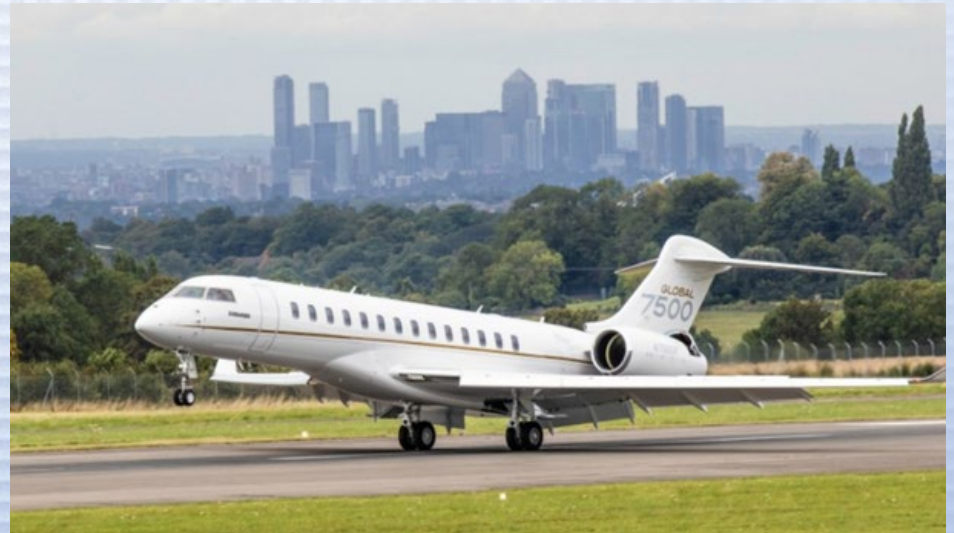
Bombardier Global 7500 with GE Aviation Passport 20 Engines
