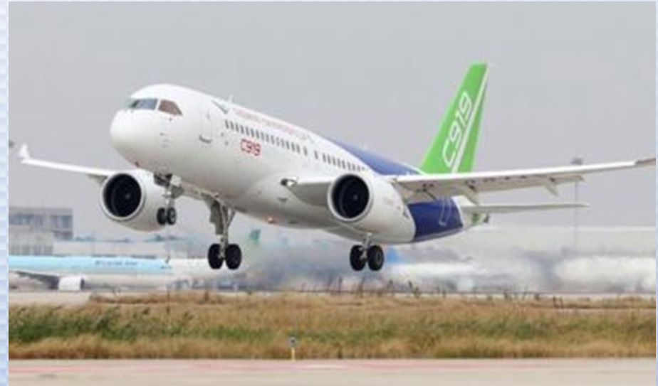
Comac C919 with LEAP-1C Engines
