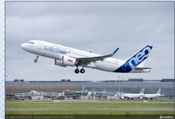
Airbus A320neo with CFM LEAP-1A Engines
