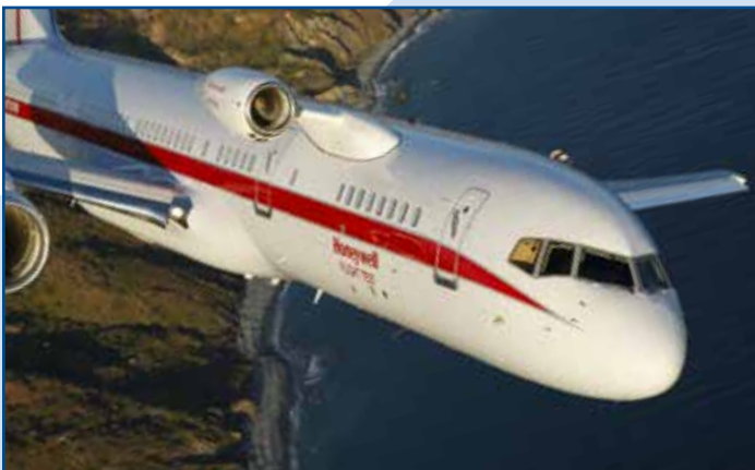
New Business Jet Turbofan Mounted on Testbed Fairing Built by Park
