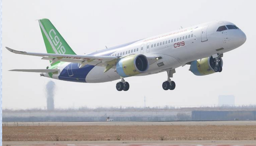
Comac C919 with CFM LEAP-1C Engines
