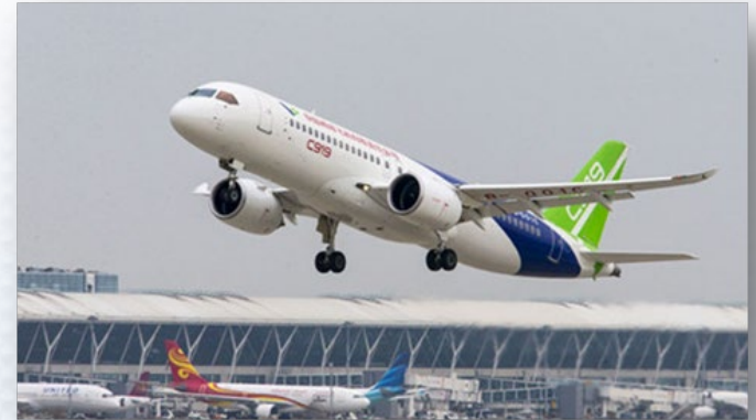
Comac C919 with CFM LEAP-1C Engines
