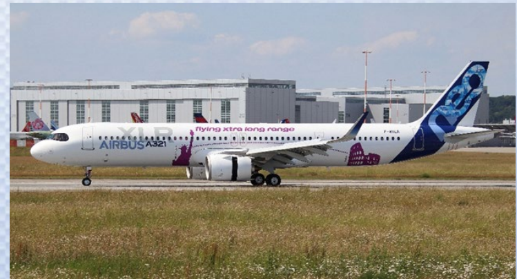
Airbus A321XLR with LEAP-1A Engines
