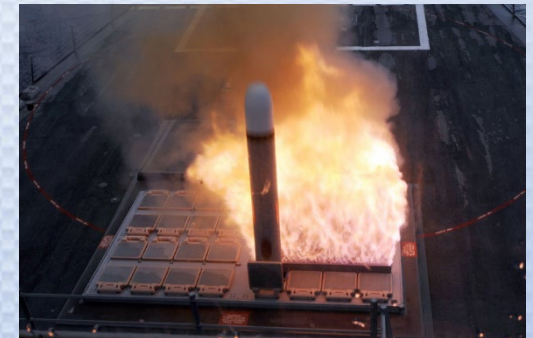
Mk-41 Vertical Launching System
