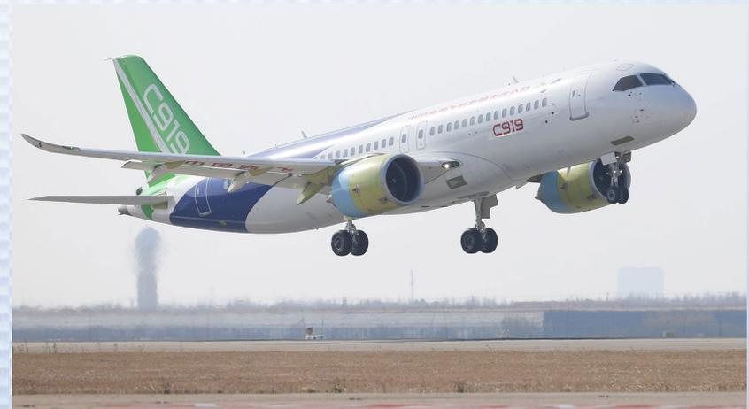
*Comac C919 with CFM LEAP-1C Engine*
