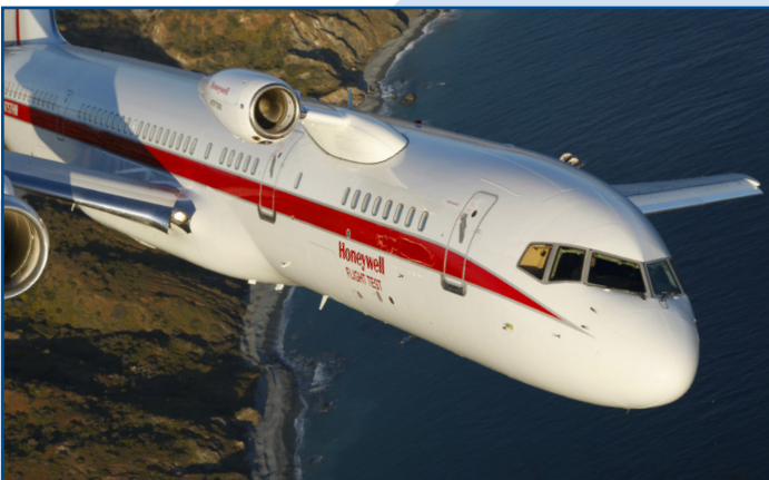
New Business Jet Turboprop Mounted on Testbed Fairing Built by Park
