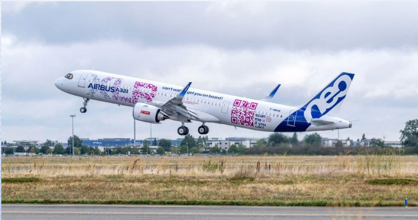
Airbus A321XLR with LEAP-1A Engines
