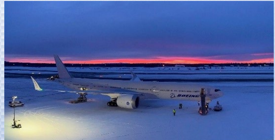
Boeing 777X undergoing Cold Weather Testing in Fairbanks, Alaska
