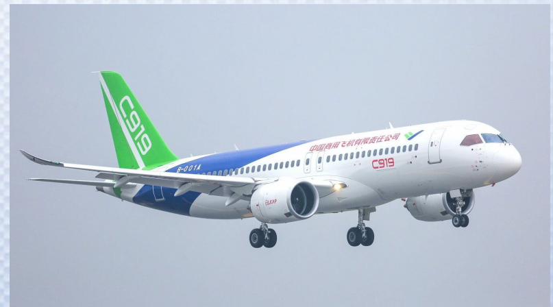
Comac C919 with CFM LEAP-1C Engine
