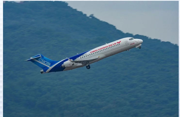
Comac C909 with GE CF34-10A Engines
